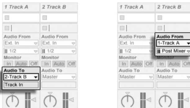
Two Ways to Route Track A into Track B.
