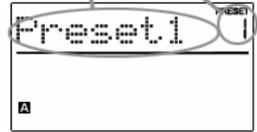
The MPK49 features different Preset banks that you can load and write to. When you turn on the MPK49, it will automatically go into Preset Mode and Preset 1 will be displayed on the screen. You can also press the **[PRESET]** button at any time to call up this mode. In Preset Mode you can load, save/copy and rename Presets – each of these functions can be accessed through the 3 different pages. You can navigate between these pages with the **[<]** and **[>]** buttons.
