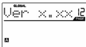
**VERSION** allows you to see what version of the operating system and firmware is currently loaded onto the MPK49.
