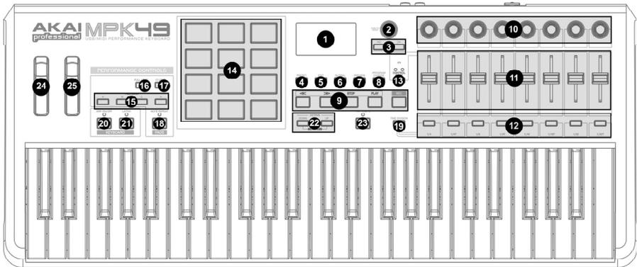
1. **LCD** – The display is used for navigating menus, displaying data, and affecting change on MPK49’s options and parameters.
