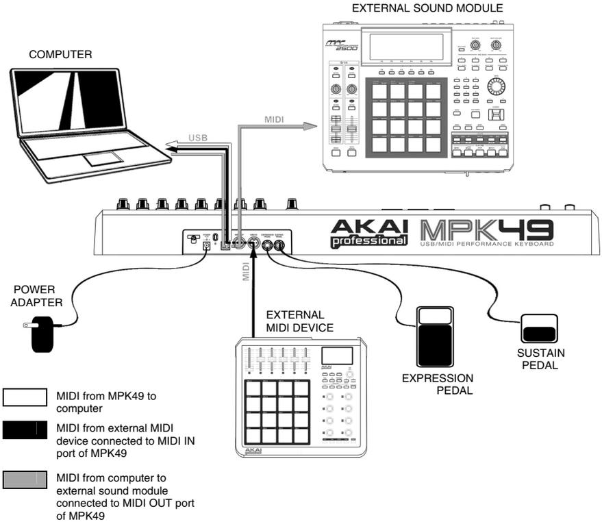
1. Connect a USB cable from your computer to the MPK49. The unit will be powered through the USB connection. Alternatively, if you do not wish to use a computer in your setup or if you wish to power the MPK49 externally, please plug in the included 6V-1A DC power adapter.
