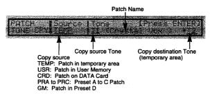
Use the VALUE knob, [INC]/[DEC] buttons, or SOUND GROUP buttons to select the copy source ("Source"). Use the VALUE knob or [INC]/[DEC] buttons to choose the Tones ("Tone") for the copy source and copy destination.
