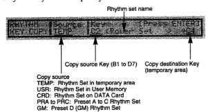
Use the VALUE knob, [INC]/[DEC] buttons, or SOUND GROUP buttons to select the copy source ("Source"). Use the VALUE knob, the [INC]/[DEC] buttons, or the keys on the keyboard to choose the keys ("Key") for the copy source and copy destination.
