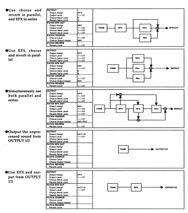
The examples here use one Tone from the Patch mode. Since the Output Level, Chorus Send Level, and Reverb Send Level can be set independently for each Tone, you can make whatever settings you need for each one when using multiple Tones. Individual settings for the Tone level are basically ignored when in the Performance mode—the level is controlled by the settings for output made for each Part. (It may be helpful to substitute PART for TONE when viewing the illustration.)
