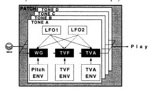
With the JV-1DBD, you can also use a parameter called "Structure" to create sounds with pairs of Tones. See "1. Patch Edit Mode" in Chapter 3 (see p. 43) for details.
