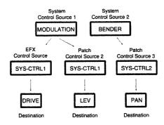
It is convenient to use System controllers when you do not need to specify controllers independently for each Patch, or when you want to be free to use any control change number as the controller.
