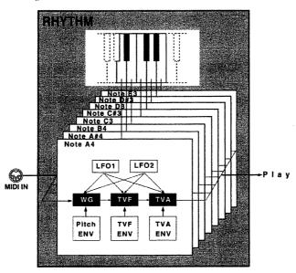
When you play keys on the synthesizer or other instrument connected to the JV-1080, you'll hear the same sound at different pitches if you're using a Patch, but if you're using a Rhythm Set then each key plays a Rhythm Tone with a completely different sound. Rhythm Tones in a Rhythm Set differ from the Tones of a Patch in a very important way — you can't combine them to create a single percussion sound.
