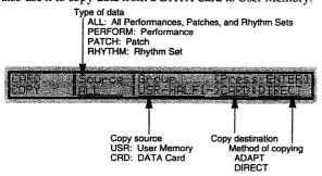
Use the VALUE knob, [INC]/[DEC] buttons, or SOUND GROUP buttons to select the type of data ("Source"), copy source and destination ("Group"), and method of copying.
