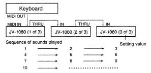
When set to "OFF," the Stack function is disabled and each JV-1080 plays in sequence all of the note messages that are received.
