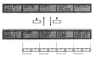
Press the FUNCTION SELECT button on the left side under the display
