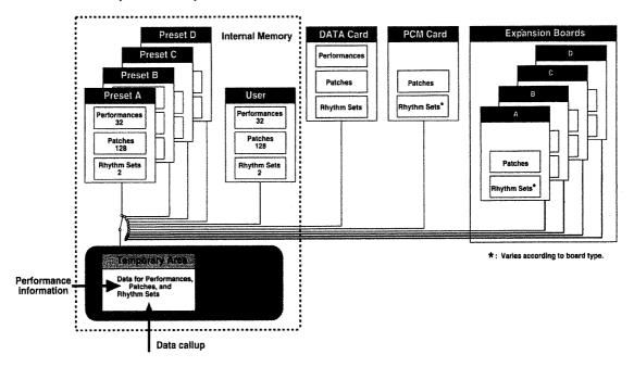
The sound data stored in these memory devices is first read into a temporary area and then played. When editing as well, the sound data called into the temporary area is changed.
